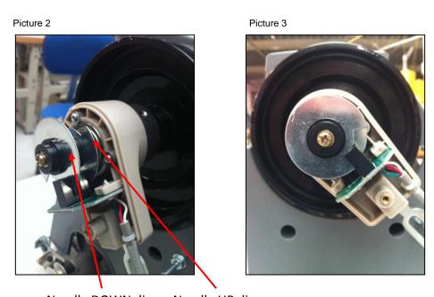
Needle DOWN disc Needle UP disc
